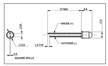
Figure 2: new led specification
