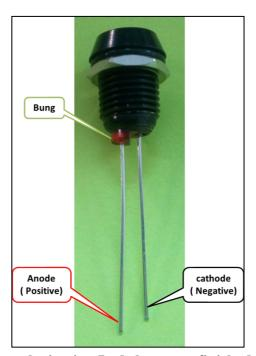
Figure 3: polarization Led shown on finished product
