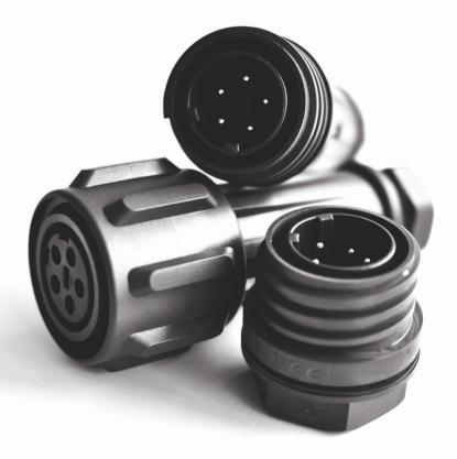
Independently tested for compliance to ATEX standards for use in Zone 2 and Zone 22 environments, the new EXP series is manufactured from a tough,high grade UL94V-0 rated Polyester material and provides environmental sealing to IP68. The ATEX coding is: Ex II 3 GD and the certificated no: Baseefa09ATEX0232X.
